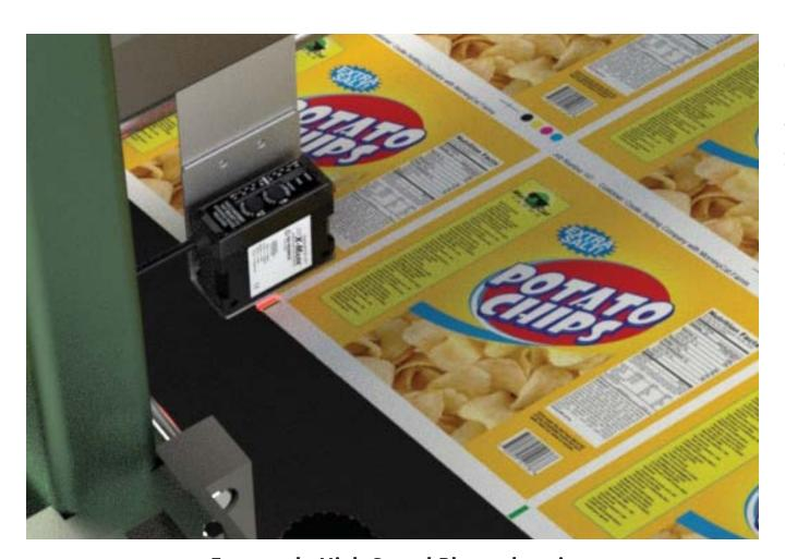
**Extremely High Speed Photoelectric Registration Sensor**
